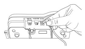
4. Place the AC Adapter cord around the strain relief.
